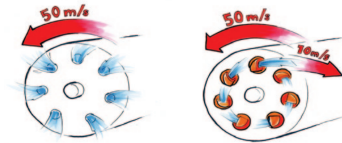
Figure 3 - Velocities at the liquid discharge
